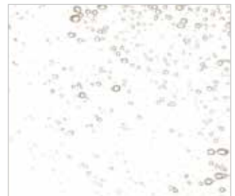
polyalphaolefin (PAO) air release: 12 seconds
