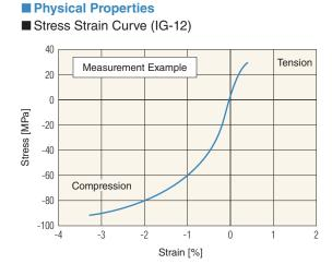
Graphite generally shows elastic-plastic deformation. The fracture behavior is different under tension and under compression, so caution must be exercised.
