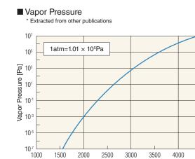
Graphite is an extremely stable material in temperatures under 2,200°C. However, the vapor pressure increases in higher temperatures and high vacuums, so caution must be exercised with regard to the accelerated wearing of graphite.
