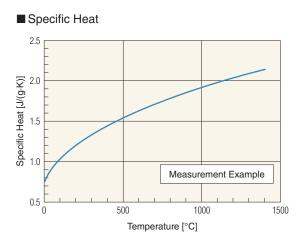
Due to the anisotropic nature of its crystals, the specific heat of graphite at room temperature stays at 1/3 of that of general solids. The specific heat value is essential in various thermodynamic functions. At high temperatures, specific heat values are similar regardless of the graphite grades.
