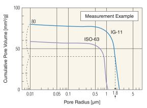
This shows the pore distribution through the mercury penetration method. The pore distribution has a close relationship with gas permeability and other unique properties of graphite. The halfway position of the cumulative pore volume indicates the average pore radius.
