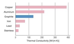
The thermal conductivity of graphite is fairly high, while the coefficient of thermal expansion is very low. These characteristics contribute to its superior thermal shock resistance. The relationship between thermal conductivity and electrical resistivity of graphite in room temperature is indicated below.
