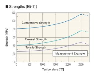
An unparalleled characteristic of graphite, which makes it indispensable in high temperature applications, is that as the temperature rises (up to 2,500°C), the strength also increases. Strength reaches levels approximately double those at room temperature.
