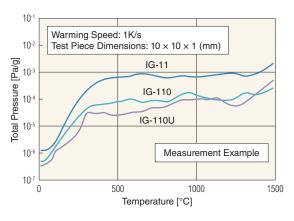
Graphite emits absorbed gas when in high temperatures. Some applications such as semi-conducting industries must use highly purified or ultra highly purified graphite, which emits less gas.
