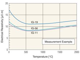
Since thermal characteristics differ from grade to grade, the coefficient of electrical resistivity must be carefully studied when selecting a grade for a heating element.
