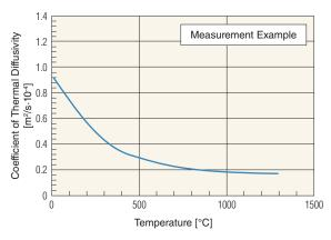
This chart shows that the higher the temperature rises, the faster the heat is transmitted. The thermal diffusivity of graphite is superior to other materials.
