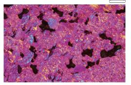
Isotropic high density graphite is different from conventional graphite in that it is isotropic and has a micro particle structure, creating a very strong and highly reliable material with a small variation. This isotropic graphite material resolves the problems associate with conventional anisotropic graphite.
