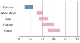
Dynamic Coefficient of Friction on a Steel Surface [Atmospheric Room Temperature]
